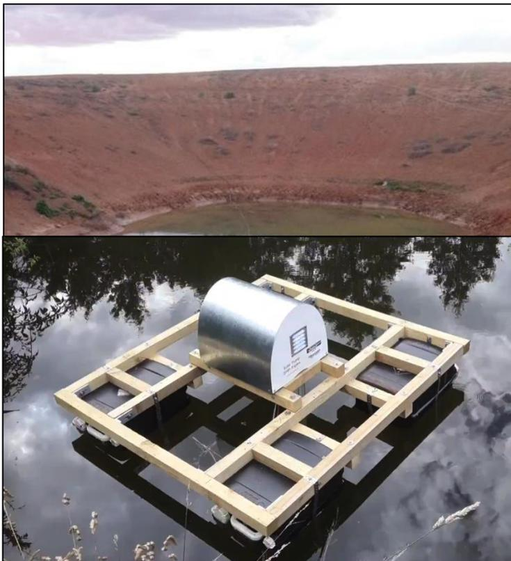
Petrol/diesel pumps are often drowned in flood events as it is not practical to put them on a floating pontoon (as they need refuelling) and are heavy. If you fail to move petrol/diesel pumps quickly during heavy rain they can get drowned in the rising water.
