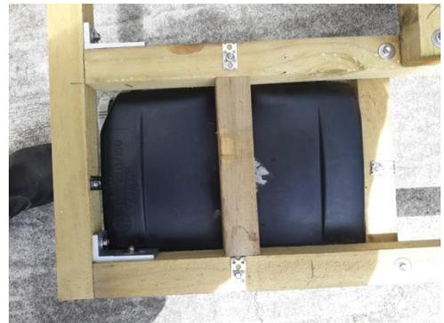
As a general rule the buoyancy of a 4 float pontoon (mass of water to fill floats) needs to be >2 times higher than the total mass. This it to ensure that should one float leak the pontoon will still float upright with the RP2 above the water line. This will then be observed and the leaking float repaired or replaced.
