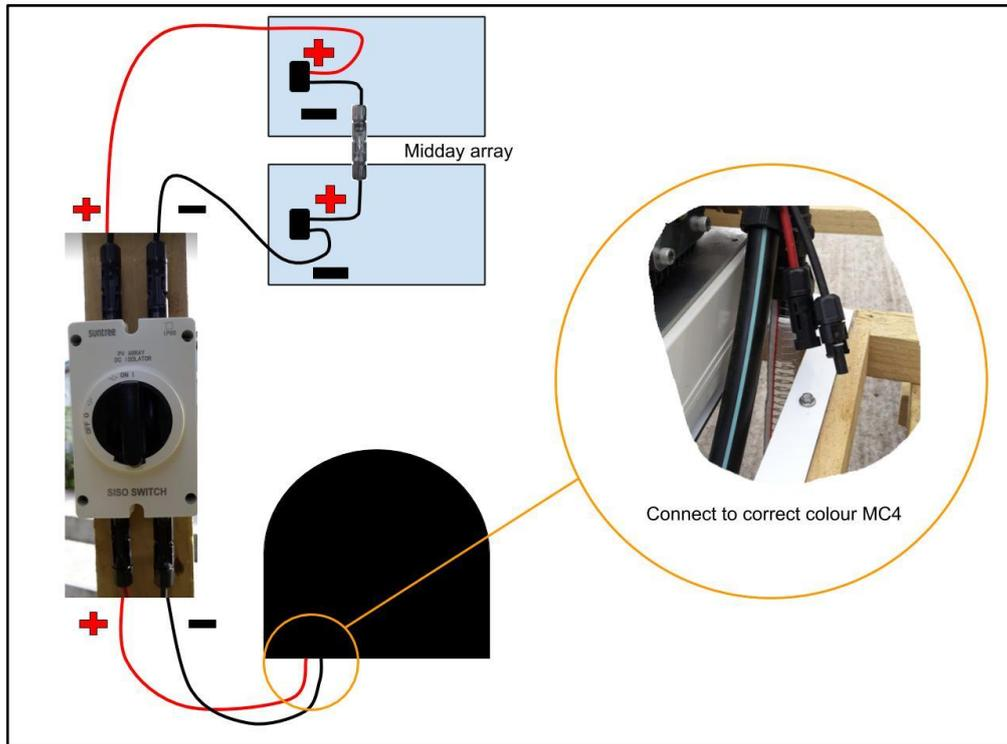
3.2.7. Wiring schematic for a 4 panel PV array
