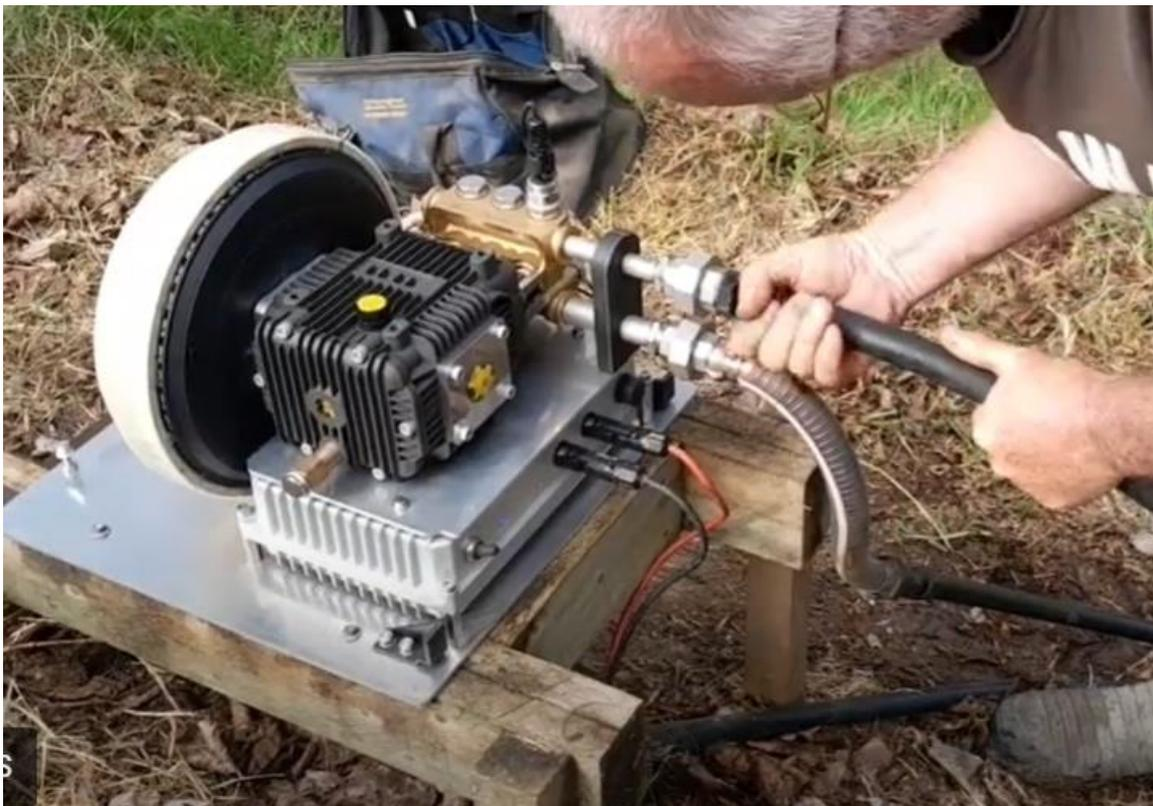
RP2 being installed (with fairing removed). Note this is in Northland NZ where frost is unlikely, the RP2 is supplied via pond water that is just above the pump location - so we have positive head on the inlet side, positive feed head is the best and most reliable option.
