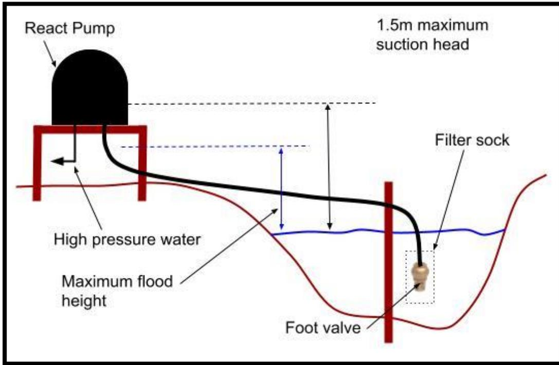
4.2.8. Submersible pump & settling tank for dirty water supplies from 1.5-50m below the RP2
