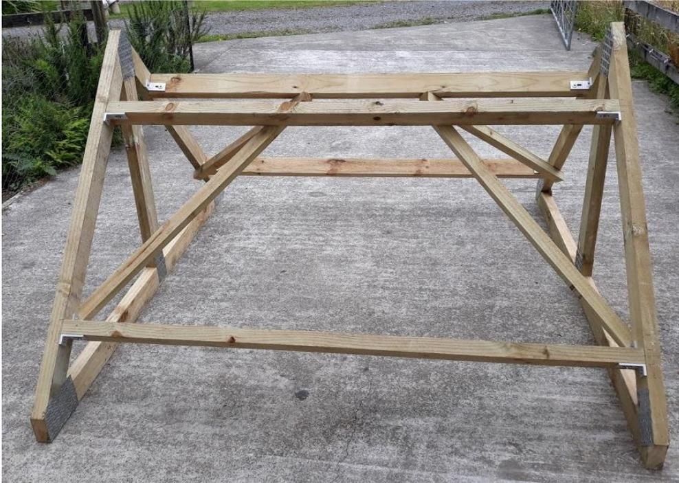
Note the four 50 x 50 x 1200mm fence battens are used for lateral bracing. It is all held together with common Tek screws, gang nail plates and angle brackets.
