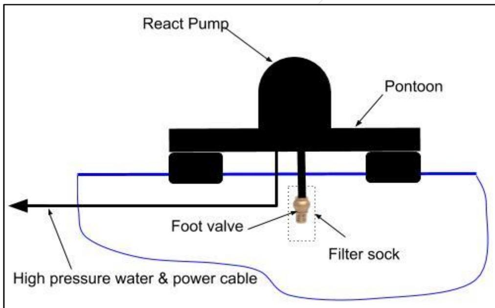
Please note that all pontoons used on streams or rivers need to be adequately secured against flood flows, wind and flood debris. For lakes and dams (that are not exposed to such risks) ropes from the pontoon and anchored to the bank are sufficient for the pontoon to maintain its set location against strong winds and water currents.
