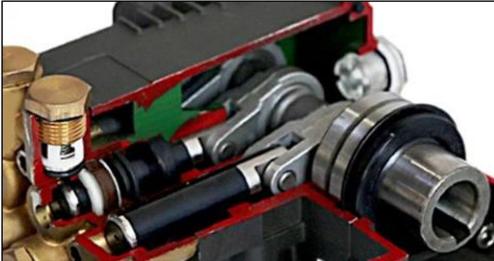
Note on the RP2 design the brass head is packed off the pump body
