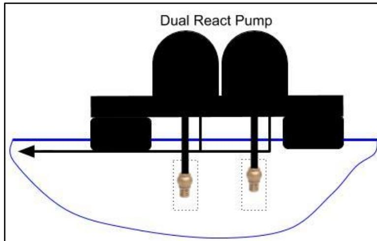
Multiple pumps can be connected to the same delivery pipe to increase your flow.
