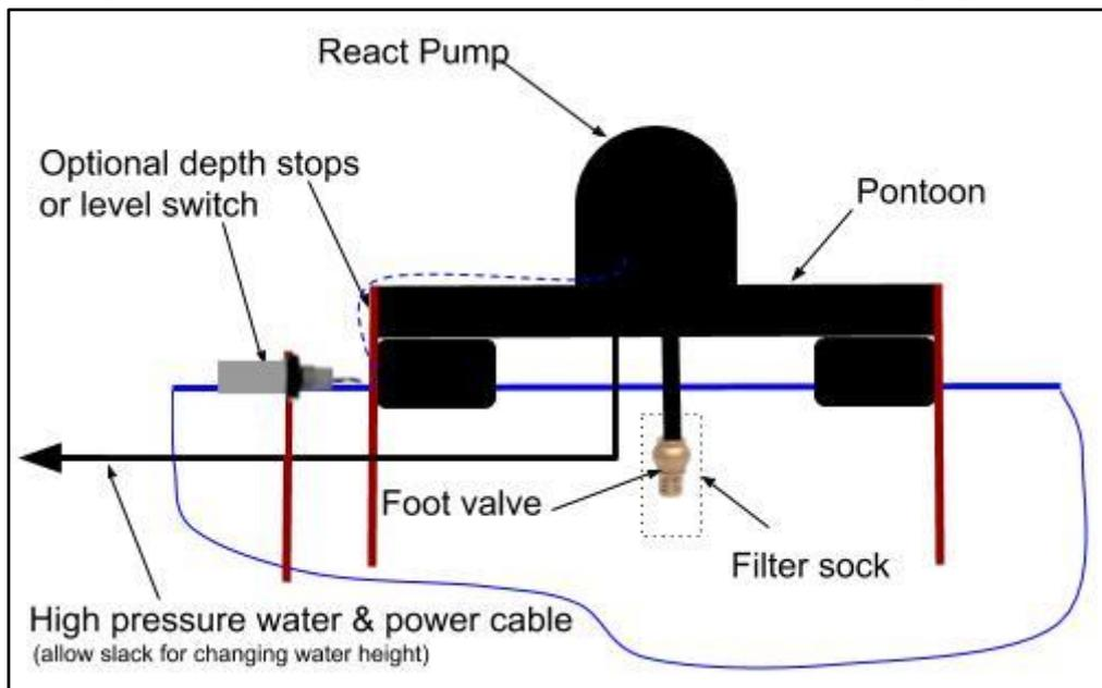
Note the pump should not be allowed to operate unless the foot valve is fully submerged.
