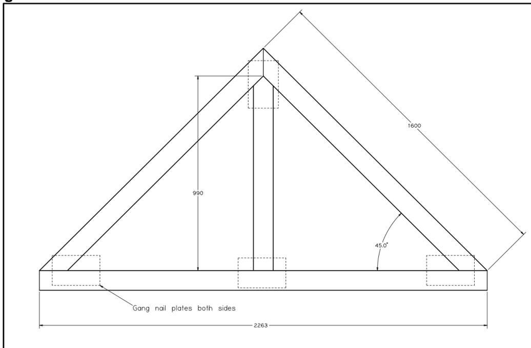
Make 2 trusses as shown from 100 x 50mm treated timber. You will also need 4 x 2m long 100 x 50mm treated timber purlins to connect the 2 trusses together as shown later.
