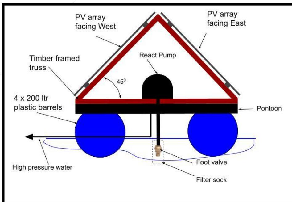
Larger lakes and dams can accommodate the solar PV array on the same pontoon as the RP2. The advantages are:
