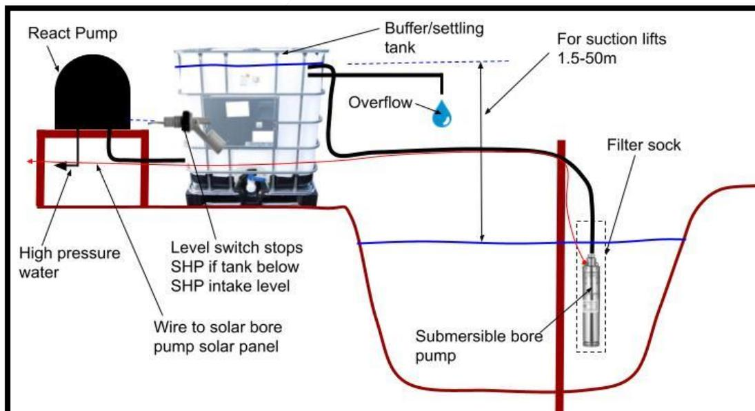
Note the buffer/settling tank and float switch will accommodate flow variations between the RP2 and the small low cost bore pump while always ensuring a positive head to the RP2. **Note:** small bore pumps with external controllers can have an external float switch added to stop the bore pump when the buffer tank is full.
