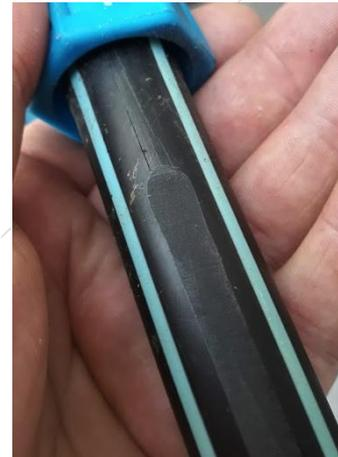
You can weaken the pipe by filing a flat on the top of the pipe plastic with a file, it will then fail at this point should the pipe be exposed to excessive pressures.
