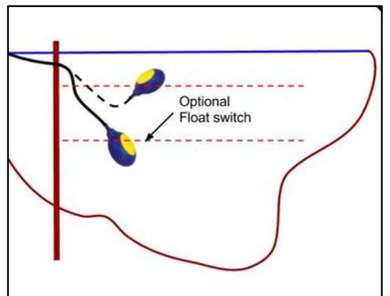
Then you can install a RP2 on a small pontoon in the middle of your pond with the suction hose set about 200mm below the surface where UV from the sun helps to sterilise the water being pumped. Design the pontoon structure to sit on the bottom of the pond before the foot valve intake hits the mud/silt level and where the RP2 turns off.
