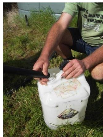
On a typical day at midday in January we measured 20 litres in 80s = 15 l/min
