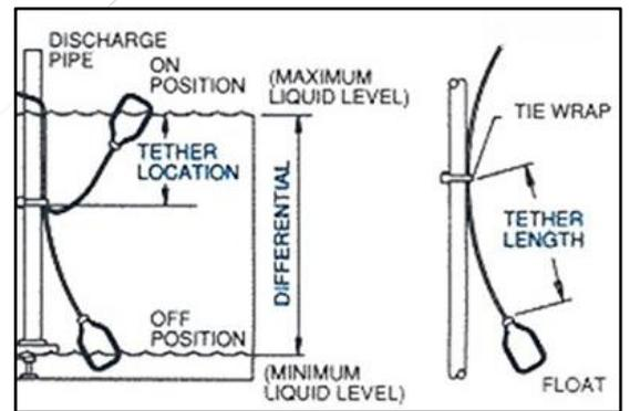
This solution will stop the pump at the lowest acceptable level of your water intake resource.
