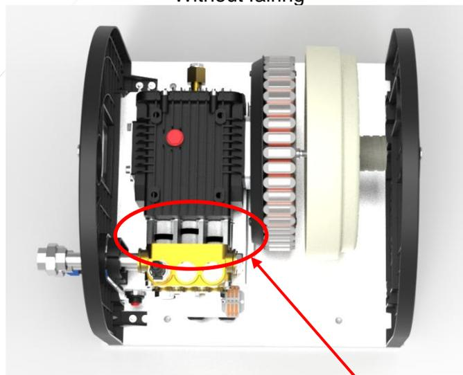
Plan view – part fairing – note the new packed head design on the RP2
