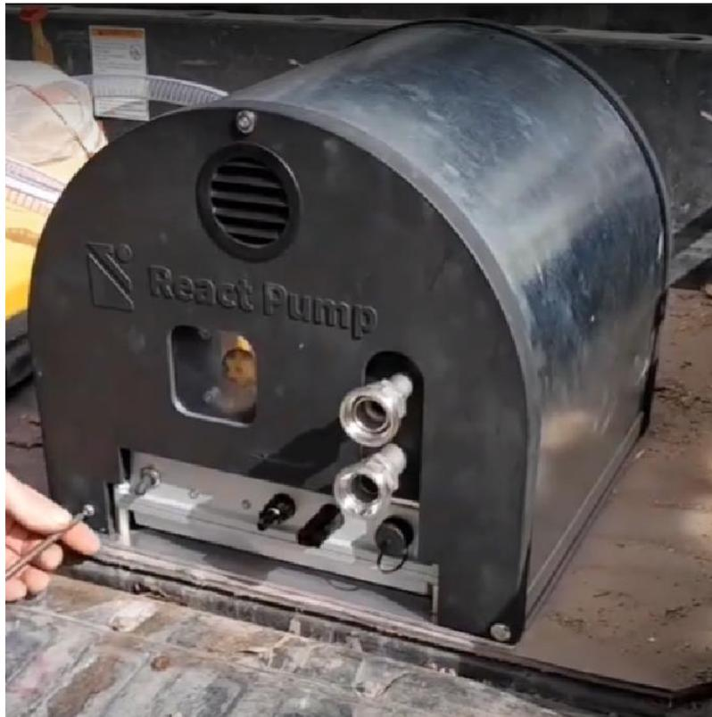
Screw to remove fairing on RP2
