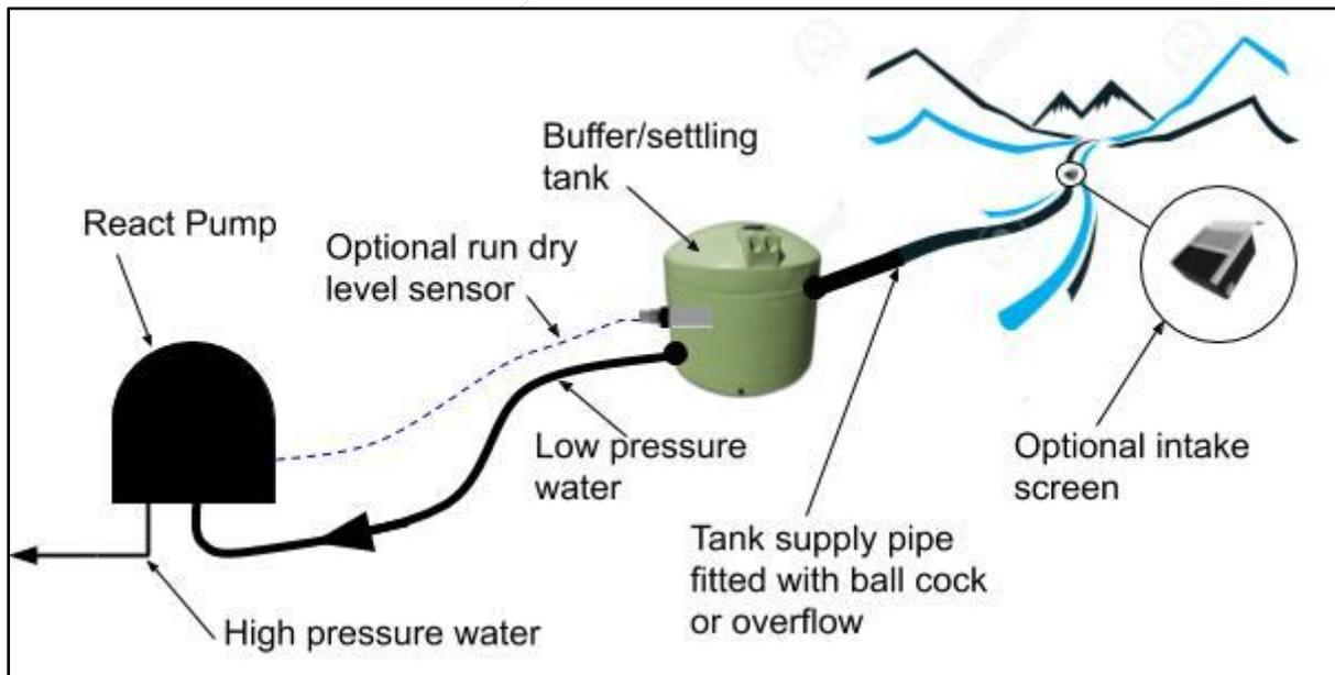
A 1mm intake screen to filter flow is advised – no foot valve is needed
