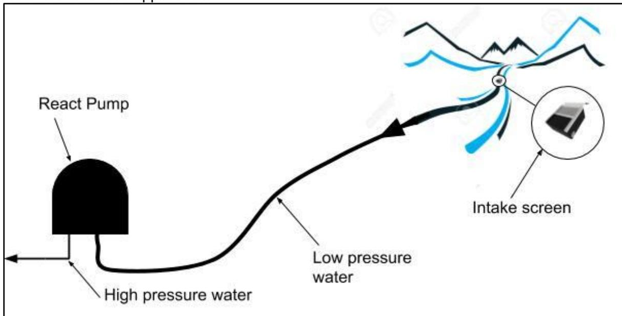
A 1mm intake screen to filter flow is required – no foot valve is needed
