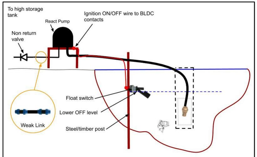
To stop the RP2 a float switch port and float is provided.
